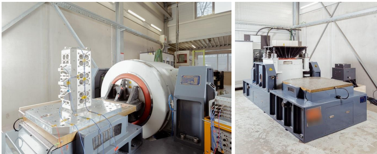
Figure 1 - 120kN Double slip table shaker : small table (left) & big table (right)
