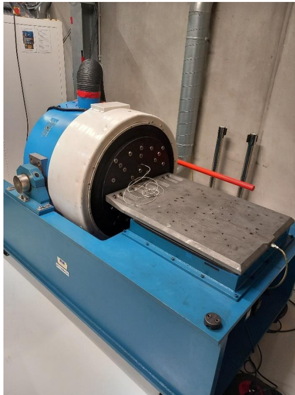
Figure 7 - 26kN large single slip table shaker
