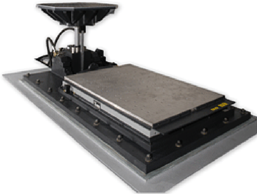
Figure 9 - 26kN large single slip table shaker
