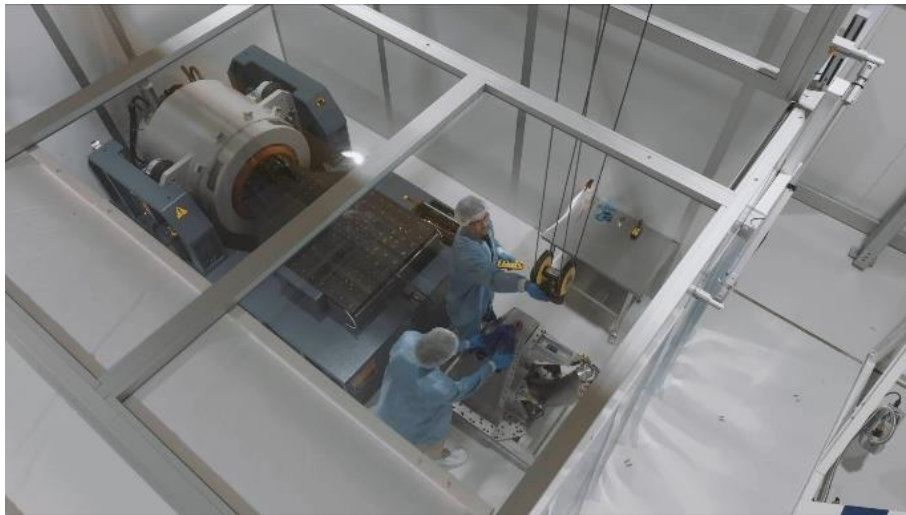
Figure 3- 120kN single slip able shaker: overhead crane access
