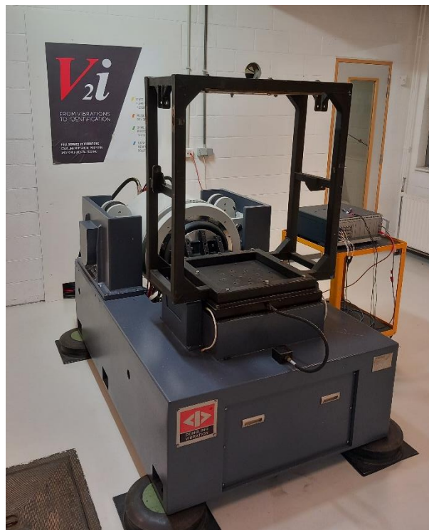
Figure 5 - 35kN single slip table shaker
