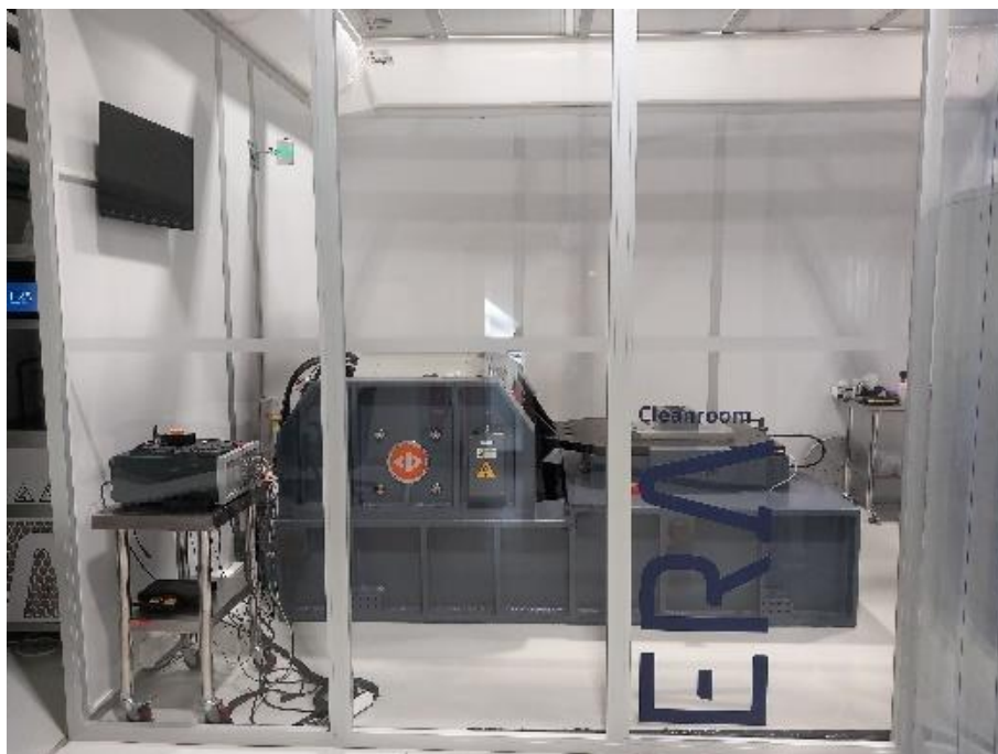
Figure 2 - 120kN single slip table shaker
